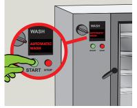
The detergent concentration should typically be 0.5% - 2% depending on level of soiling Select Automatic wash and press start/stop key.
