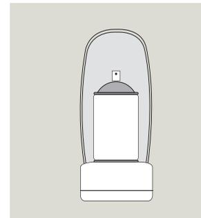
**3** Open dispenser by pressing the button located on top of the unit. Remove the lid from the spray can and place inside the dispenser.
