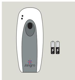
**2** Place batteries into dispenser. Ensure the unit is switched off when replacing batteries or aerosols.
